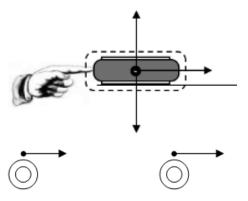
The arrows above the images of the puck are intended to convey the changing speed of the puck. In this case the length of the arrows represents the speed of the puck and the direction the arrows point represents the direction the puck is moving.
