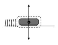
The most important thing to understand about this situation is that the puck will, as long as the forces remain balanced, travel at the same speed in a straight line. Nothing is required to cause the puck to keep moving. An unbalanced force would be required to cause it to go faster or slower, and/or an unbalanced force would be necessary to change its direction. But in the absence of an unbalanced force, the puck will continue to move in a straight line at a constant speed.
