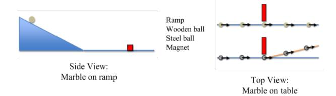
Use a ball on ramp to create a constant velocity along the tabletop for a rolling ball. The wooden ball rolls past a magnet and continues to travel in a straight line. The steel ball rolls past a magnet and is pulled 'off path' with a slight change to the path.
